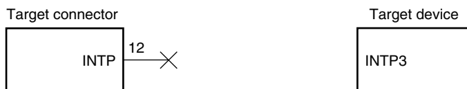
Figure 20-3. Circuit Connection for the Case Where QB-MINI2 Is Used Only for Programming
